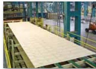
Sheets of veneer go to grading and processing
